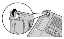
**2** Press the tabs in the direction of the arrows (①), then remove the wall mounting adaptor (②).
